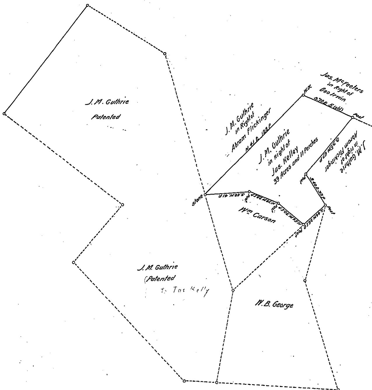
Survey of the James Kelley warrant dated Jan 29 1817. Original Survey July 15 1817. Part patented is shown by dotted lines, the parts unpatented are marked on plan Wm Carson and W. B. George and J. M. Guthrie part asked to be patented is marked J. M. Guthrie in right of James Kelley.
